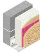
One-Coat System with Lath or Mesh
